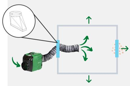
To create a positive pressure: Locate the Raptor outside the internal space. Fix the 3m x 250mm flexible ducting to the unit. Feed the ducting in through a window; the fishtail can be used to reduce the opening. When switched on, the Raptor will force clean air into the room and force contaminated air out through windows and vents. The high airflow will maintain a positive pressure environment.
